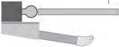
Actuator support bracket mounted horizontally on hinge post
